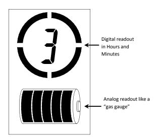
The RealTime™ LCD provides on-the-fly remaining run time estimates in 15 minute increments as well as providing remaining capacity information using the traditional "gas gauge" approach. In this way, the LCD provides two different methods of determining battery capacity.
